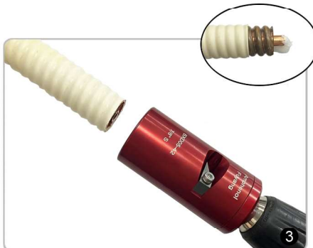
Insert the cable into the trimming tool. Select the low speed on the drill or 400~600 RPM on a variable speed drill. Trim the cable until no further debris generated.
