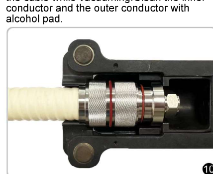
Make sure the connector and cable both lay flat in the compression frame.
